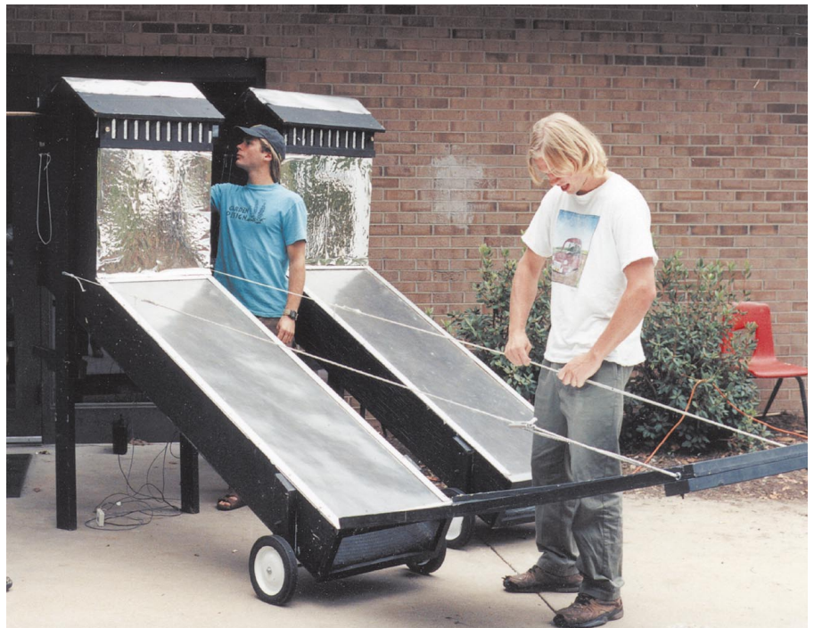
Above, Photo 4: Setting the front reflector angle.
